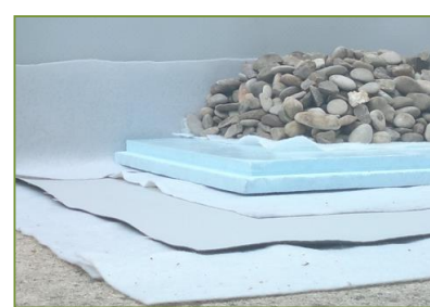
Inverted flat roof
