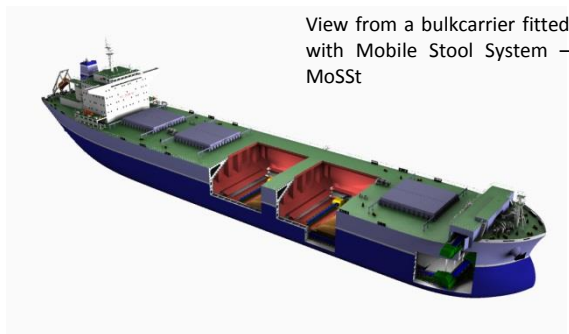
View from a cargo hold fitted with Mobile Stool System - MoSSt
